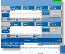
Closed-Loop Control provides up to 4 control loops. Use control outputs to control line equipment such as Puller, Extruder, Air Pressure, Take-Up and other devices.
