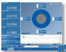
Home Page displays cross-sectional view of tube and pipe concentricity, and enables you to precisely monitor product dimensions, reel length and line speed to reduce start-up time and scrap for quality production. Easily customize the Main Menu to the way you work.
